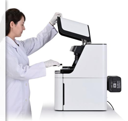
ECLIPSE Ji fits standard laboratory benchtops, has built-in vibration dampening hardware, and works in bright environments. There is no need for dedicated space or dark rooms to perform efficient imaging assays.
