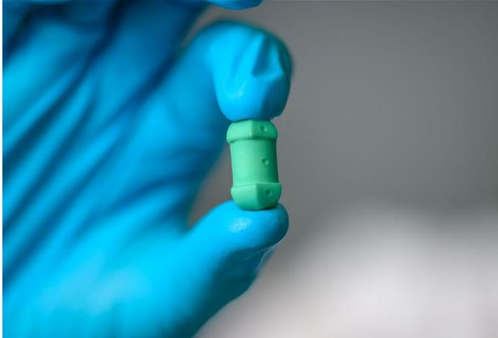
The single-use, factory-calibrated pill is simply dropped into the shake flask culture. Circulating with the medium, it measures dissolved oxygen continuously.
