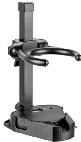
The MPS is positioned in the adapter, underneath the shake flask and optically reads out the DO signal, transmitted by the DO Sensor Pill.
