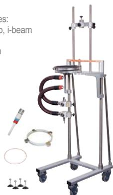
**Important:** Hoses to connect the Reactor-Ready Pilot framework to your thermoregulator are NOT included. You will require hoses with an M30x1.5 female connection or appropriate adapters. See listing for hoses, adapters and suitable thermoregulators.
