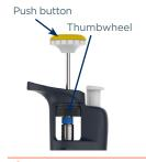
Figure 4 Location of push button and thumbwheel
