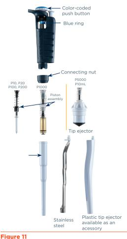
Disassembled PIPETMAN®, with different piston assemblies
