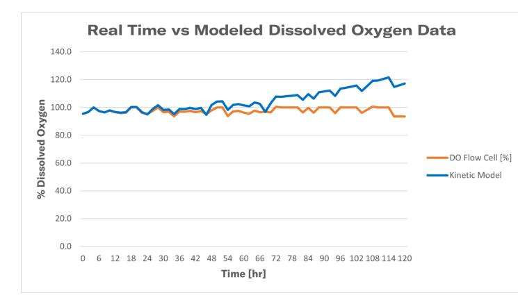
Fiber optic sensors reported approximately 5% higher, on average, than the values predicted by the kinetic model (based on OCR from static culture studies) highlighting that the cells are not consuming oxygen as fast as originally thought.
